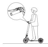
6 Press the brake lever to brake, and gently press the rear fender to assist the brake.
