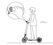
5 Press the THROTTLE button to speed up. Do not ride too fast.
