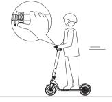
4 Press the THROTTLE button slightly on your right hand to start and rotate the handle to turn
